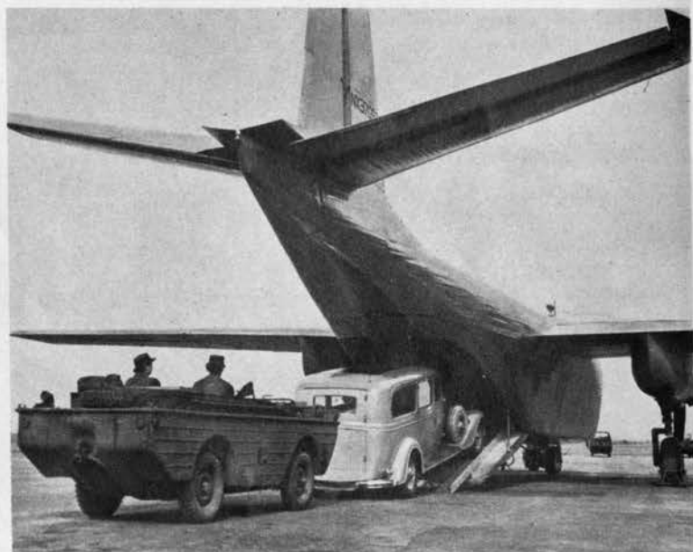
Cargo is loaded through a ramp hatch under upswept tail. The Conestoga carries more than five tons in jeeps, ambulances or fighting men.
